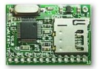
µALFAT-TF is an OEM board of µALFAT<sup>™</sup> chip with TransFlash (micro SD) card connector. It has very small dimensions which makes it ideal for small data logger. This OEM board is one of the smallest OEMs with high performance file system abilities , about 1" by 1.4"!
